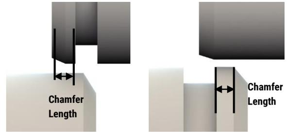
Figure 2.12: Example of Chamfer Length and Extrusion Gap
