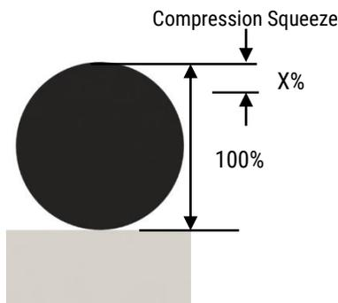
Figure 2.2: Important measurements in relation to compression ratio
