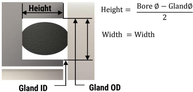
Figure 2.5: Face Gland Seal important measurements and calculation.
