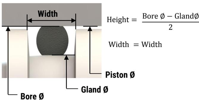
Figure 2.4: Piston Gland Seal measurements and calculation.
