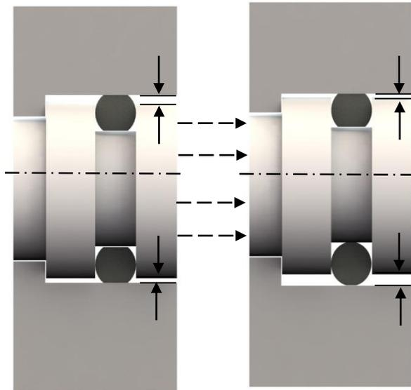
Figure 2.11: Concentricity and Diametric Clearance
