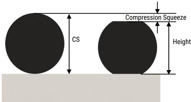
Figure 2.1: Important measurements in relation to compression squeeze
