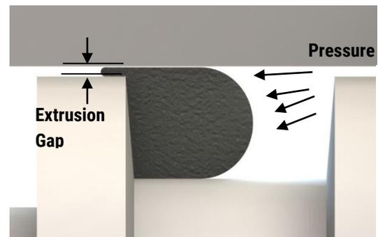
Figure 2.10: Example of Extrusion Gap
