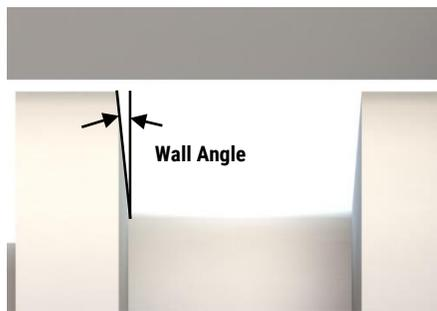
Figure 2.7: Example of groove wall
