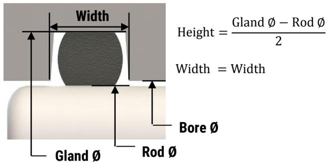
Figure 2.3: Rod Gland Seal important measurements and calculation.
