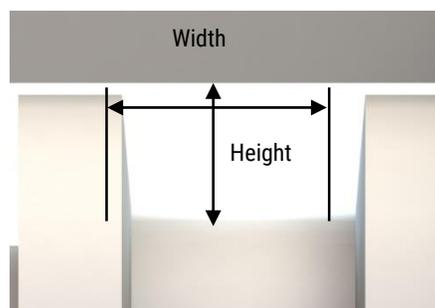
The following target gland fill recommendations take into account several hardware and O-ring related factors including but not limited to thermal expansion, volume swell due to fluid exposure and the effect of tolerance stack-ups.
